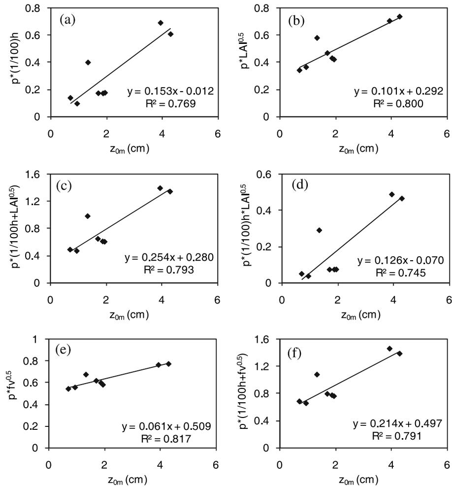
**Fig. 3.** The scatter plots between  $z_{0m}$  calculated with the sonic anemometer observational data and characteristic factors of the roughness elements.
