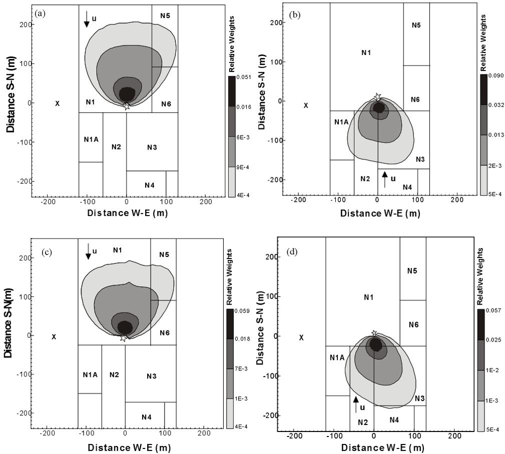
**Fig. 1.** The footprint of the eddy covariance system at northerly and southerly wind directions of the Xiaotangshan Experiment (northern sub-plot) overlays on the land cover map. Arrows denote wind direction. Stars denote the location of the apparatus with a coordinate of (0, 0). The longest isopleth determines the source area of a 90% level that limits an area that contributes up to 90% of the sensed fluxes by the instrumentation. (a, b: 1–31 May 2005; c, d: 1–10 June 2005).
